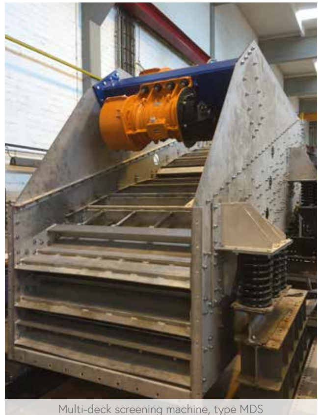
Multi-deck screening machine, type MDS made of stainless steel
