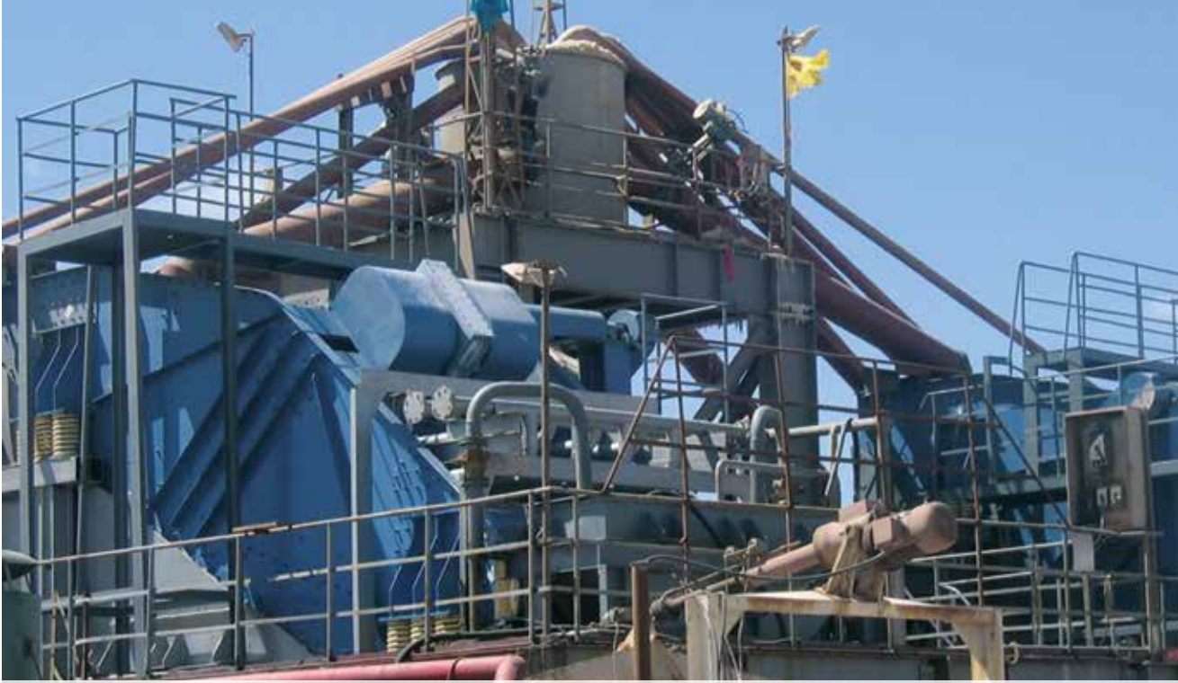
Gear-driven screen, type BHG, banana screening machines used for the screening of potash salt in China
