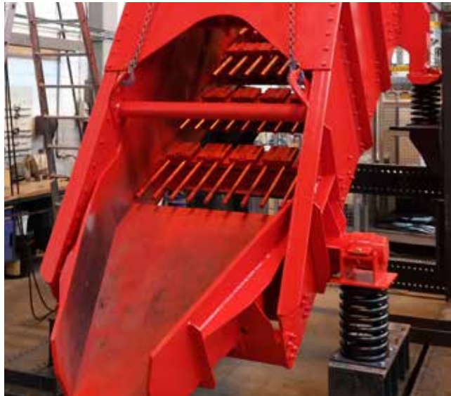
Linear-motion screening machine, type HR
