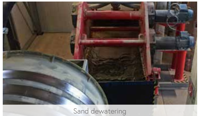
Low-pressure dewatering screening machine, type DWS-UE
