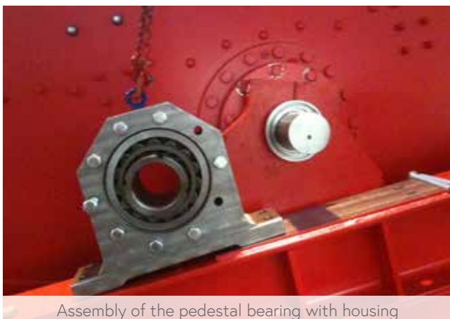
Excenter screening machine, type VS
