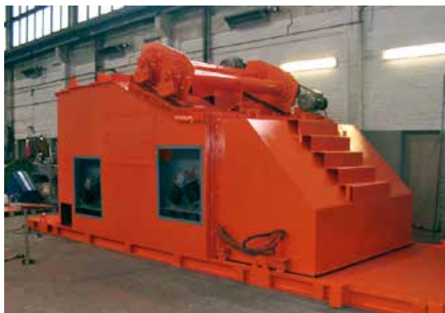
Hot standard screening machines, type HN
