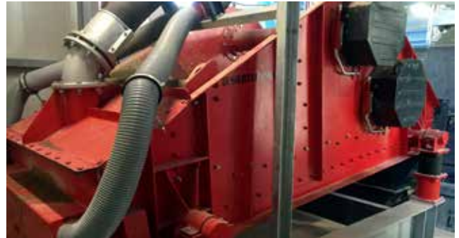
Low-pressure dewatering screening machine, type DWS-UE
