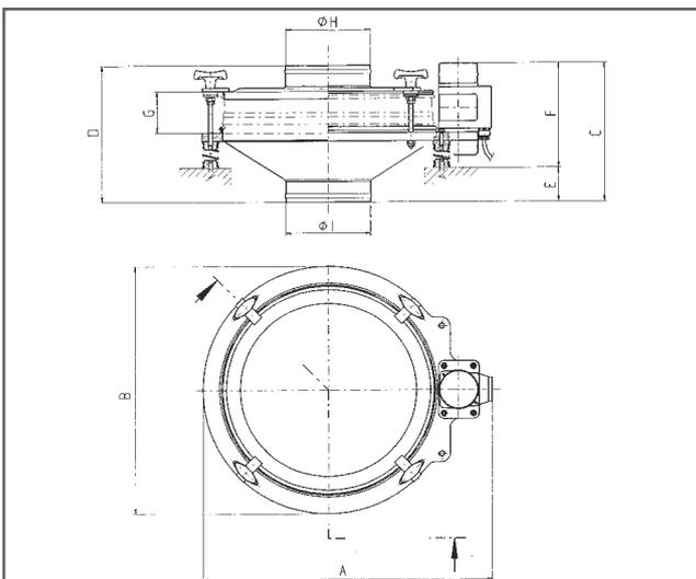
This gyratory motion allows a highly efficient and effective screening process with only one motor, thereby keeping operating cost low. Due to its compact dimensions, the machine can easily be integrated into any production process.
