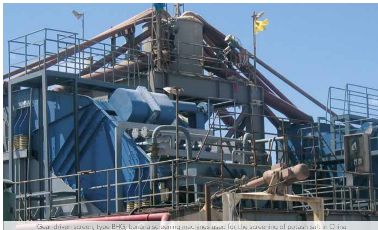
Gear-driven screen, type BHG, banana screening machines used for the screening of potash salt in China
