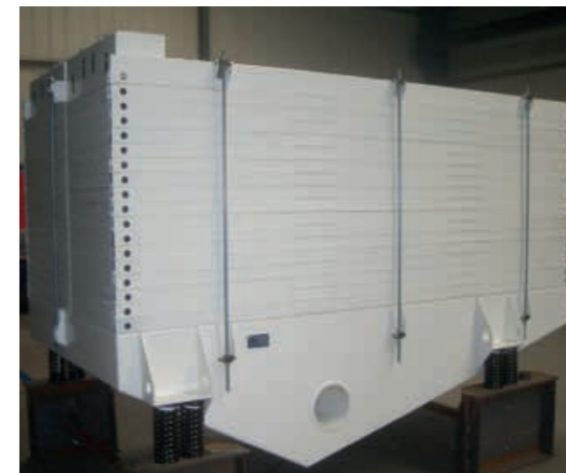
Production machine MHR 20/28/XVII (2 IIX) width 2000 mm, length 2800 mm with 17 decks in two screen units
