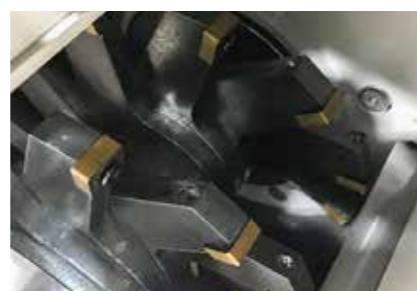
Rotor: Cutting mill design
