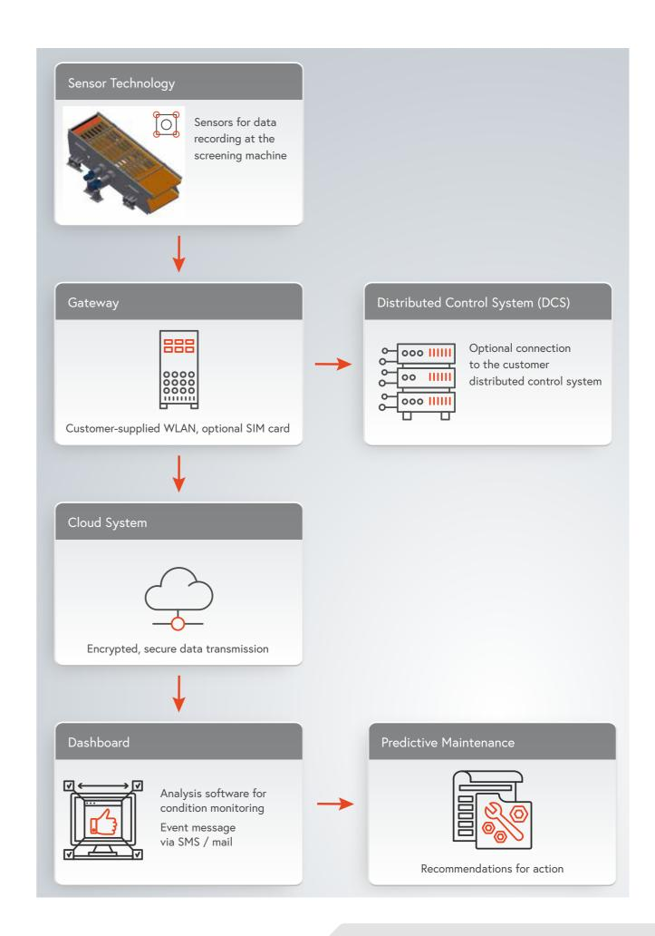
Remote Advanced Monitoring - SIEBTECHNIK TEMA - Remote Advanced Monitoring
